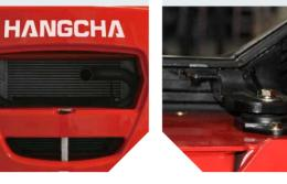
There're four levels shock absorption applied to reduced the vibration from the road to the driver. The damping pad is applied reduce the vibration, Like between the steering axle and the chassis, The engine, torque convertor and the chassis, the overhead guard and the chassis. And the suspension seat is another vibration reduction.
