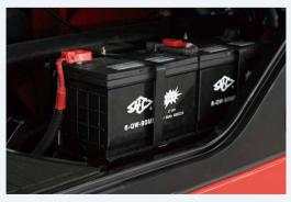
The battery is located above the fuel tank, there's battery box and adiabatic plate between them to prolong the battery's workling life.
