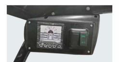
Interactive instrument: The instrument adopts LCD display with four interactive buttons, and has one CAN bus communication function. The communication protocol is compatible with CANopen and SAE J1939 standards.
