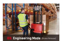
When truck is down, release the brake to move the unit manually.
